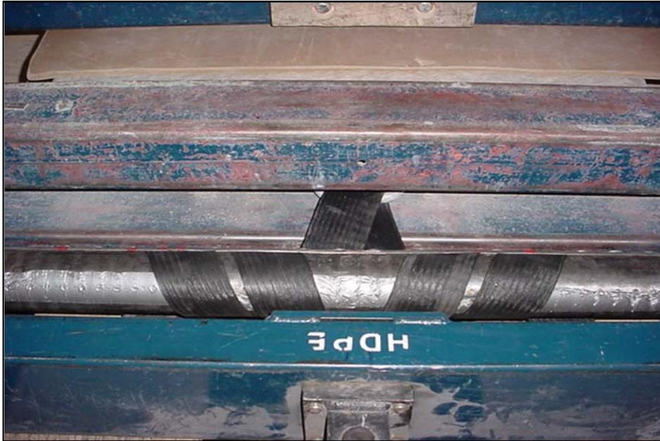
Figure 2: Photograph of connection detail and ParaWeb polyester strap in the connection test apparatus.
