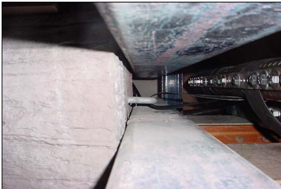
Figure 3: Photograph of Rosetta block unit with the back of block configuration in the connection test apparatus.
